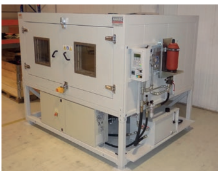
Test bench for pressure pulsation
